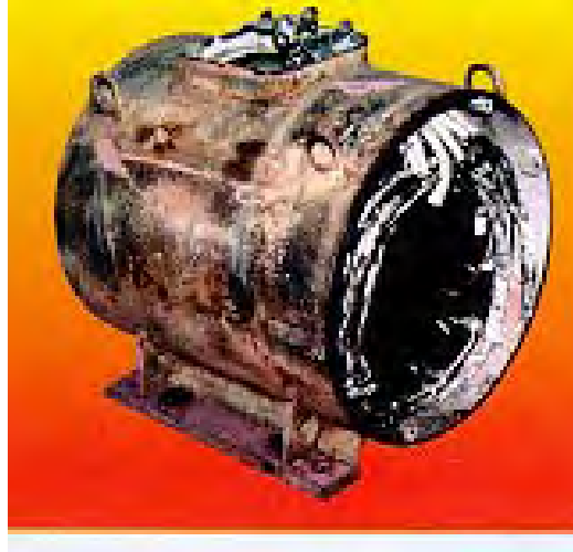
Figure 2: Burned Out Rolled Steel Stator
