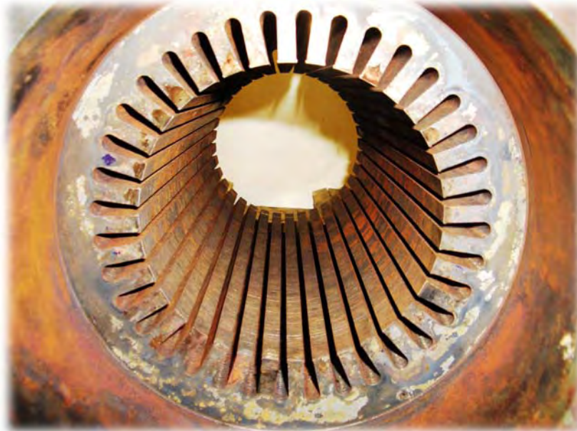
Figure 1: Burned Out Stator Core
