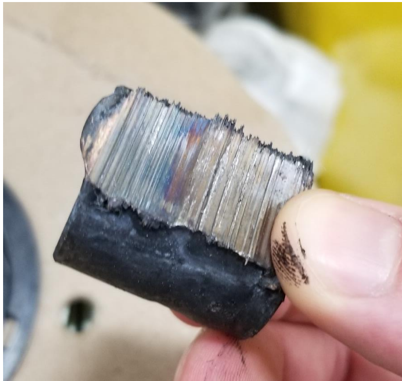
DE Bearing Roller, Evidence of Ineffective Lubrication or Starvation
