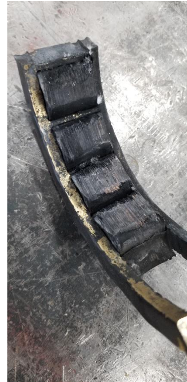
DE Bearing Rollers and Cage, Evidence of Ineffective Lubrication or Starvation
