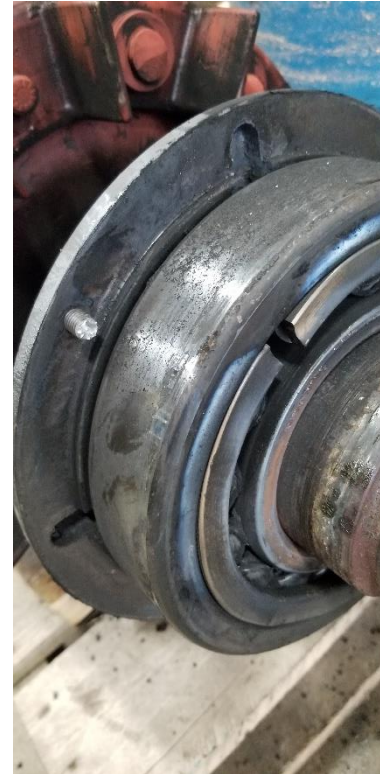
DE Bearing Failure
