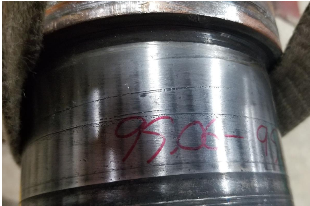
Porosity Marks on DE Journal, Evidence of Metal Spray
