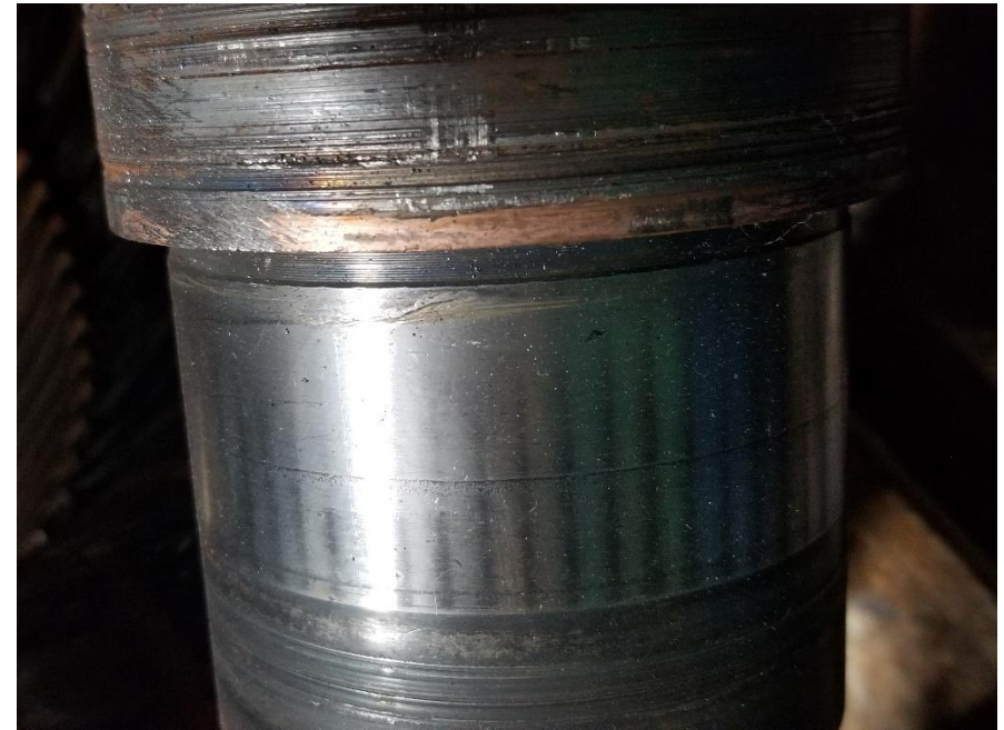
DE Shaft Journal Fretting from Ineffective Oversized Interference Fit
