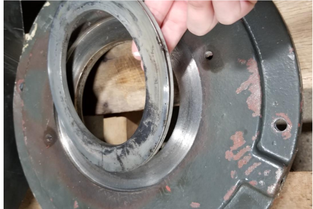
DE labyrinth and exterior bearing cap with felt seal
