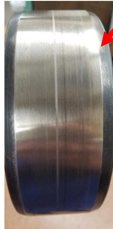
Scratch Marks on DE Inner Raceway (more prominent on output shaft side)
