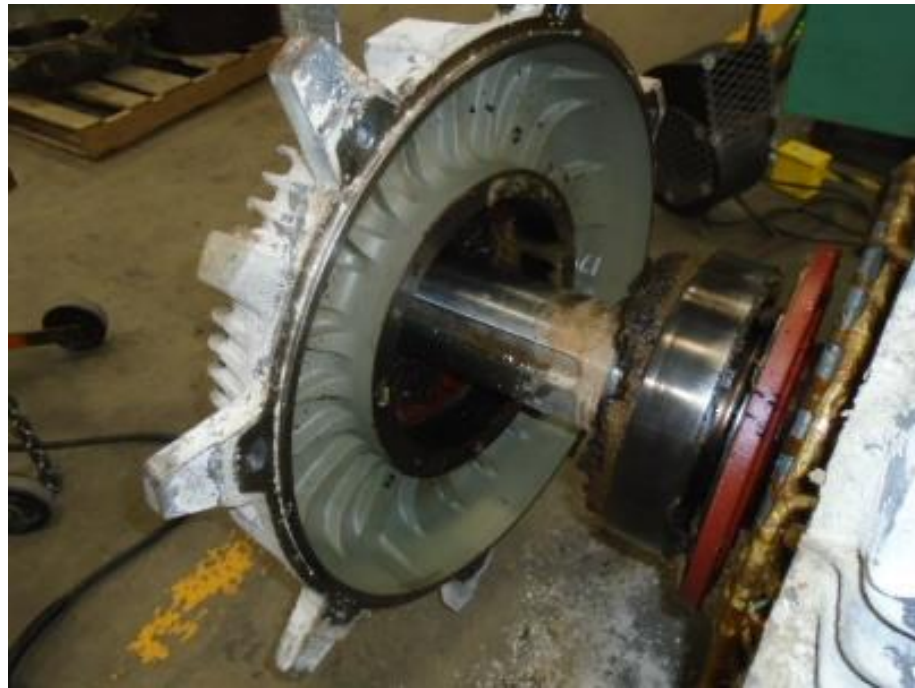
Drive End Bearing Housing Removal
