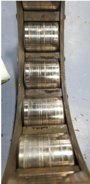
Scratch Marks on DE Bearing Rollers
