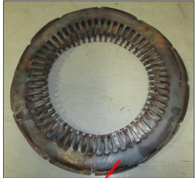
Burned out 100 HP Laminations
