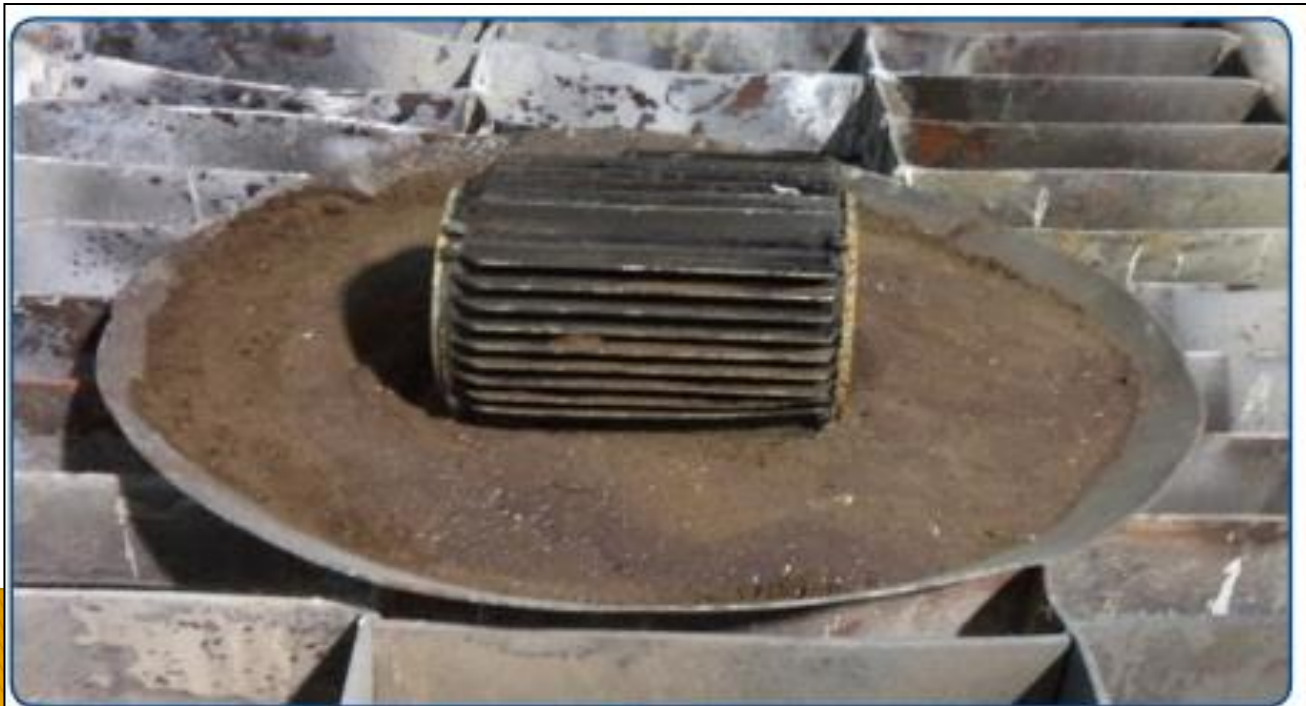
Figure 1. Aluminum frame and stator in pan of sand.
