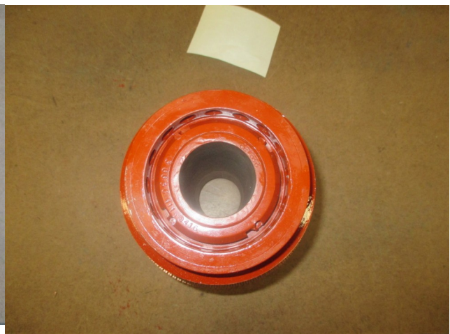
Figure Eleven: Rebuilt commutator, view of front of spool and commutator
