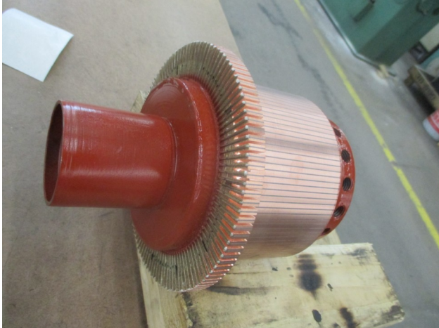
Figure Six: Rebuilt commutator, angular view of riser
