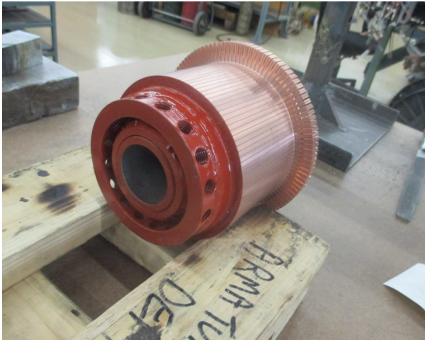
Figure Eight: Rebuilt commutator, angular view of front with new insulation
